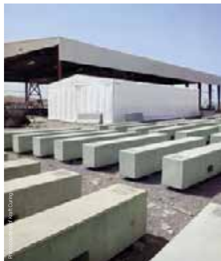
An outdoor curing enclosure can help create an optimal curing environment for precast products by maintaining appropriate temperatures and humidity levels.
