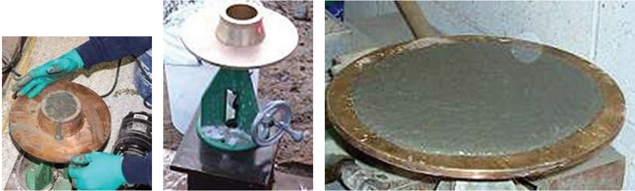
Figures 8 – The plastic flow of each batch is determined in accordance with ASTM C230.
