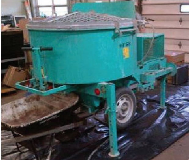
Figure 2 – Small (14-50 bags mixer) (Photos courtesy of Lafarge)
