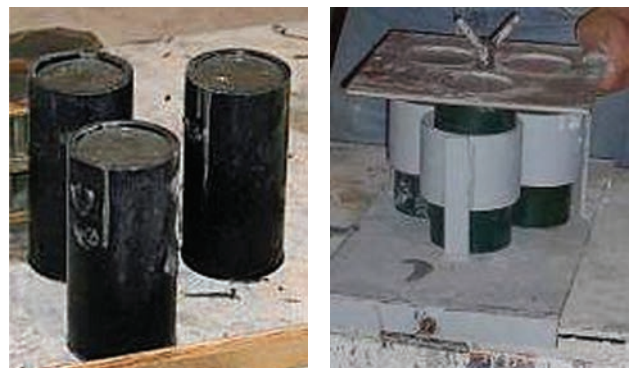
Figures 9, 10 – (left) UHPC compressive strength cylinders; (right) vibration of UHPC compressive strength cylinders
