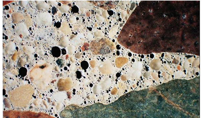
Microscopic photo of concrete showing air bubbles
