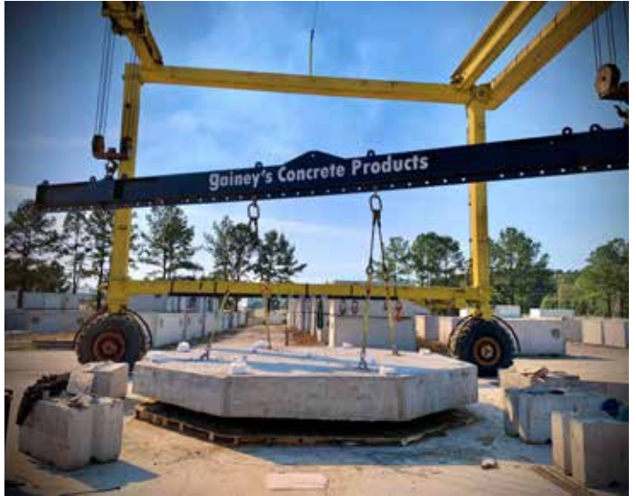
Left: A false floor is constructed inside the form to match the slope of the existing foundation underneath. Right: The completed slab with anti-slip surface finish is ready to be delivered and installed.
