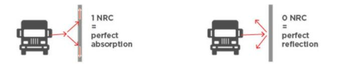
Noise wall performance is rated by two coefficients: Noise Reduction Coefficient (NRC) and Sound Transmission Class (STC). The STC determines the amount of noise energy transmitted through the wall material. The NRC determines the amount of energy absorbed by the way material and the amount of energy reflected back towards the source.
