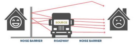
Both of the above scenarios are prime examples of where an absorptive noise barrier system would be much more effective as they actually reduce reflections.
