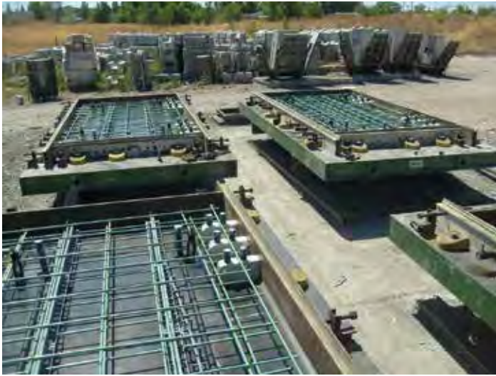
Figure 7-3. Individual, adjustable-width forms.
