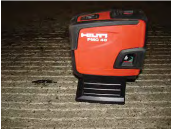
Figure 8-9. An example right-angle laser device for laying out perpendicular transverse saw cut lines.
