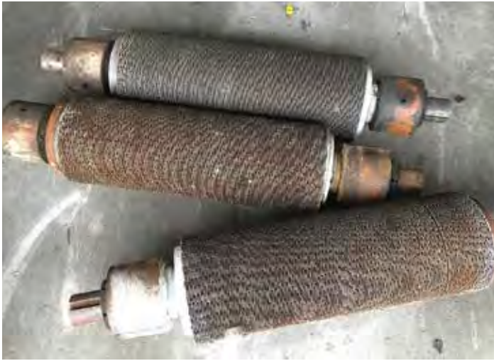
Figure 11-21. Closely spaced saw blades can be seen in this photo of a diamond profile grinding head.
