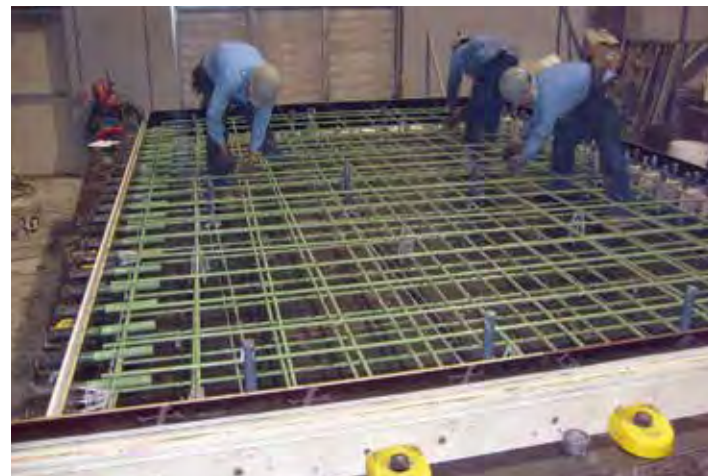
Figure 7-13. Adjustable side rails for producing general panels of any size or shape.
