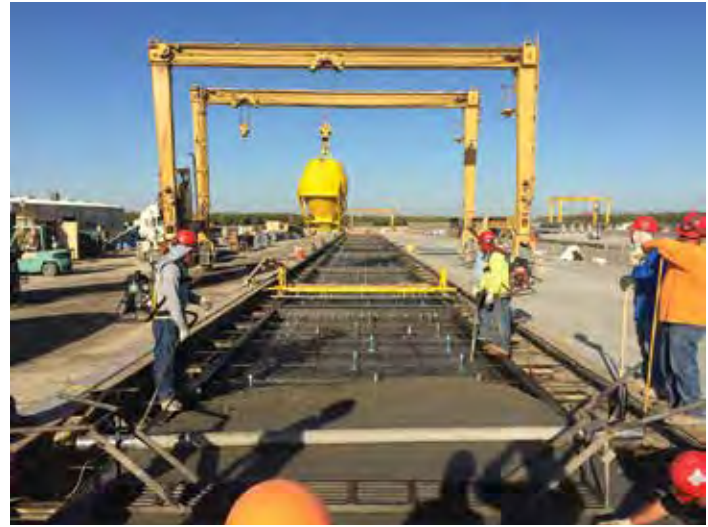
Figure 7-4. Long-line prestressing beds with adjustable end rails.
