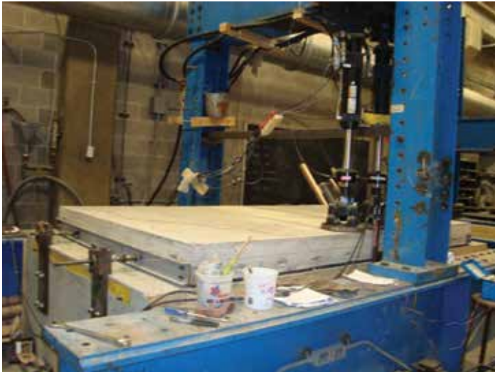
Figure 4-30. Photo and schematic of University of Pittsburgh lab-based accelerated loading pavement test stand.
