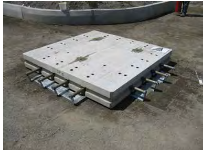
Figure 2-20. Super-Paver RUP system.
