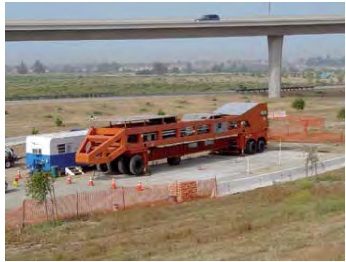
Figure 1-12. Heavy vehicle simulator testing jointed precast pavement panels in Fontana, Calif.
