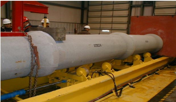
Joint Shear Test Condition C1628 /C497
