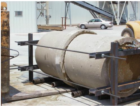
Simple 1 Piece Joint Test Setup
