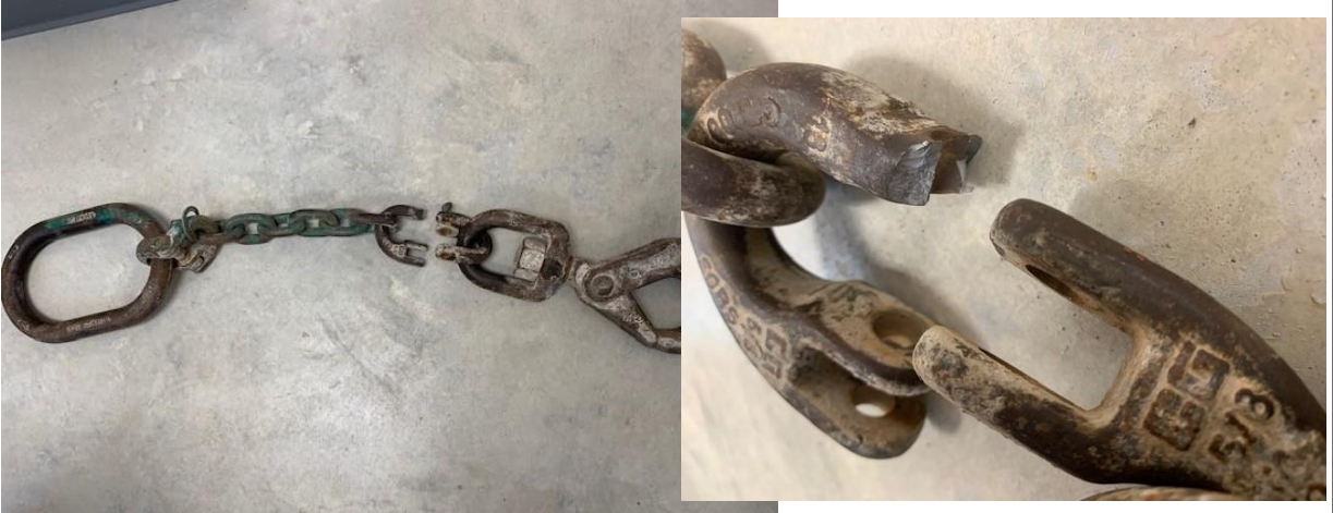
The pin holding the connecting link together sheared.
