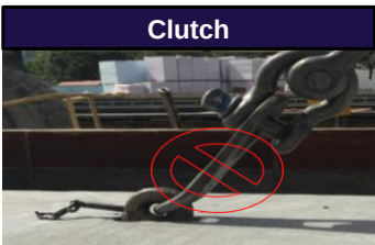
This example shows a clutch bail that is bent beyond the manufacturers' allowable tolerance
