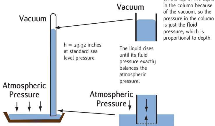
atmospheric pressure. The denser the liquid used, the lower the height of the column. In initial experiments, liquid mercury (Hg) was used, and the corresponding column height was found to be 29.92 inches of mercury. (If water had been used, the column would be 408 inches – 34 feet – high.) The following relationships can be used to convert atmospheric pressure between the units of inches of mercury (in Hg) and pounds force per square inch of area (psi):
