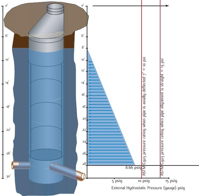
Does the Pressure Differential Exceed the ASTM C 923 Pressure Rating?
