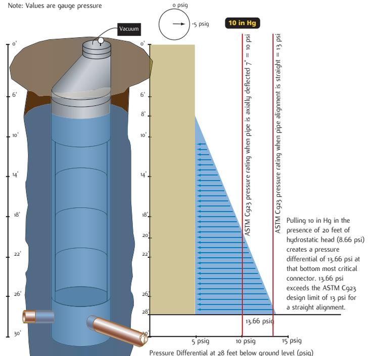
Pulling 10 in Hg in the presence of 20 feet of hydrostatic head (8.66 psi) creates a pressure differential of 13.66 psi at that bottom most critical connector. 13.66 psi exceeds the ASTM C923 design limit of 13 psi for a straight alignment.
