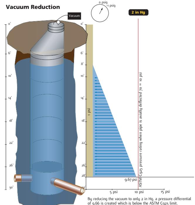
By reducing the vacuum to only 2 in Hg, a pressure differential of 9.66 is created which is below the ASTM C923 limit.
