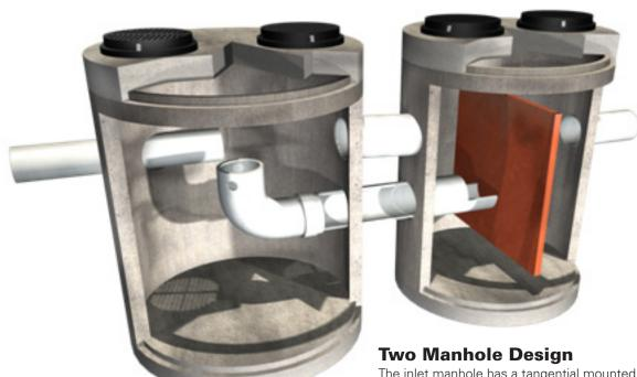
The inlet manhole has a tangential mounted inlet pipe that creates a swirl flow pattern, which improves flow distribution and reduces turbulence, thus enhancing sedimentation settling. Proper sizing essentially offers a complete removal of sandy sediment. The elbow pipe configuration in this particular design conveys flow to the outlet manhole where floating debris is retained by using an underflow baffle.
