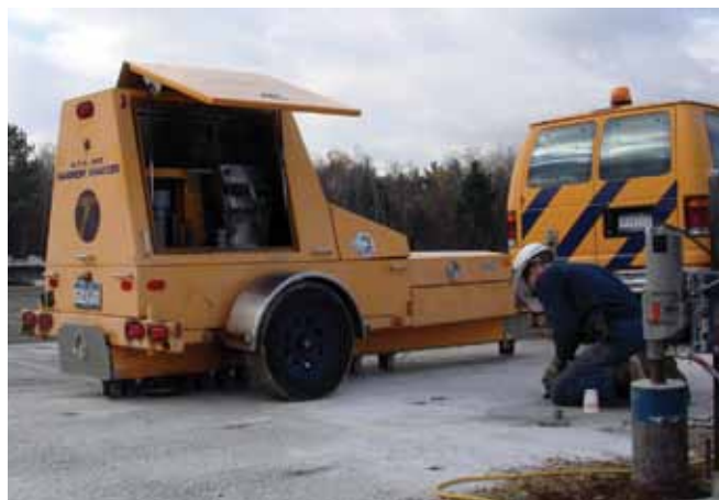
Figure 13: Falling weight deflectometer testing device
