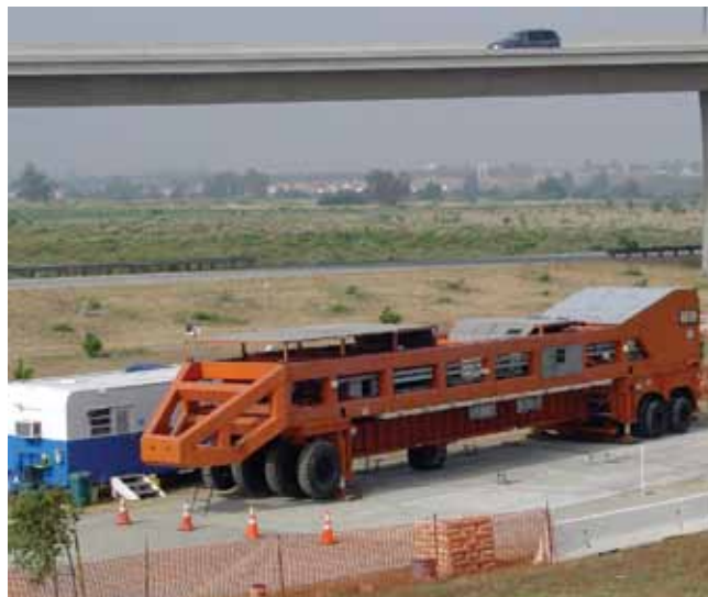
Figure 14: Heavy vehicle simulator testing device
